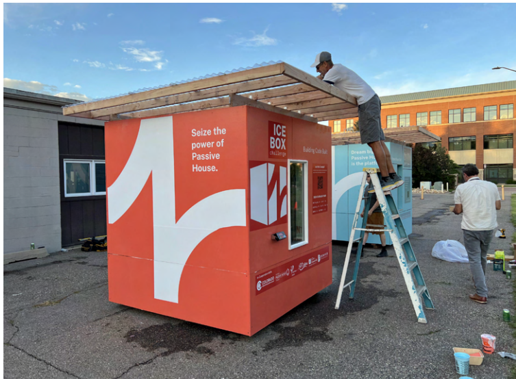
In the “Ice Box Challenge,” two rooms compete on which can keep 2,000 pounds of ice coldest the longest, one built to Passive House standards, and a conventionally designed room. The Passive House room wins by showcasing its superior ability to retain space cooling and keep out heat from outside. Image credit: The Passive House Network
